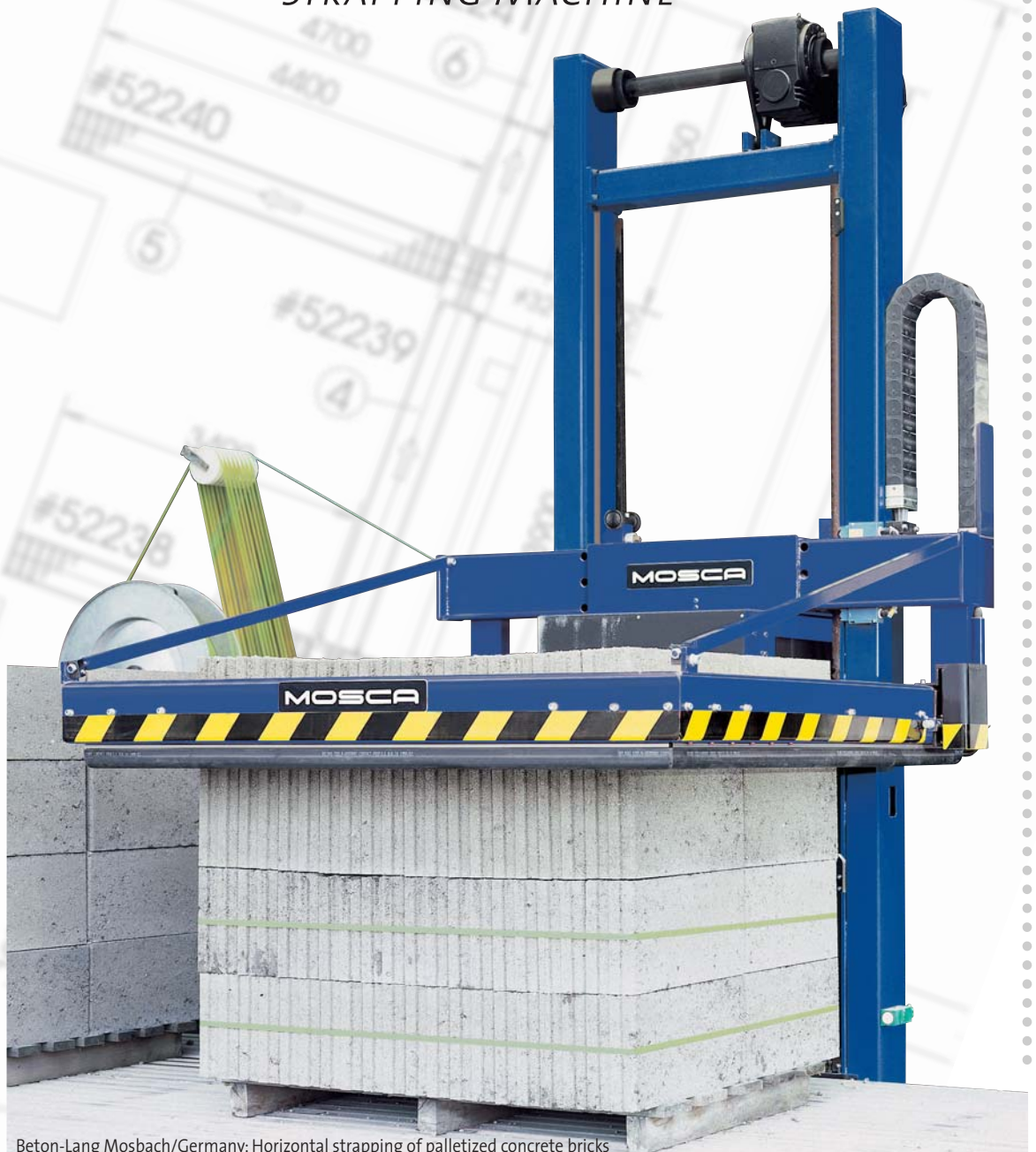
Beton-Lang Mosbach/Germany: Horizontal strapping of palletized concrete bricks
